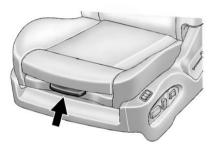
Adjust the manual leg extension by pulling up on the lever, and then pulling or pushing on the support to lengthen or shorten it. Release the lever to lock it in place.
